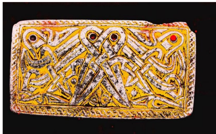
Figure 29 - Elemental mapping of gold (yellow), tin (white), and silicon (red).
